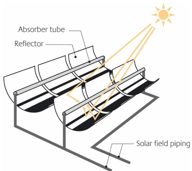
Picture 1 - Functional principle of the parabolic trough
