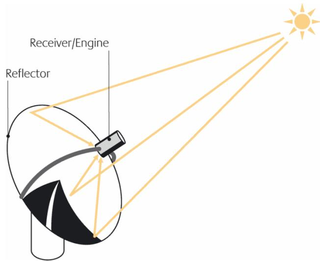
Picture 6 - Functional principle of the solar dish
