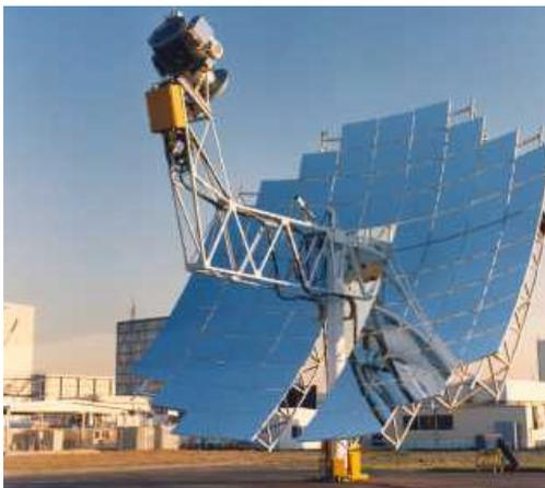
Picture 8 - Solar parabolic dish
