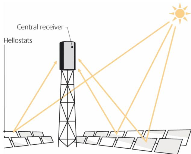
Picture 4 - Functional principle of the solar tower
