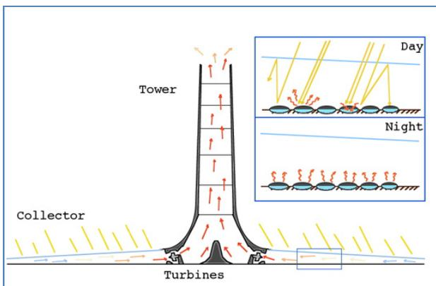
Picture 10 - Functional principle of the Solar Tower
